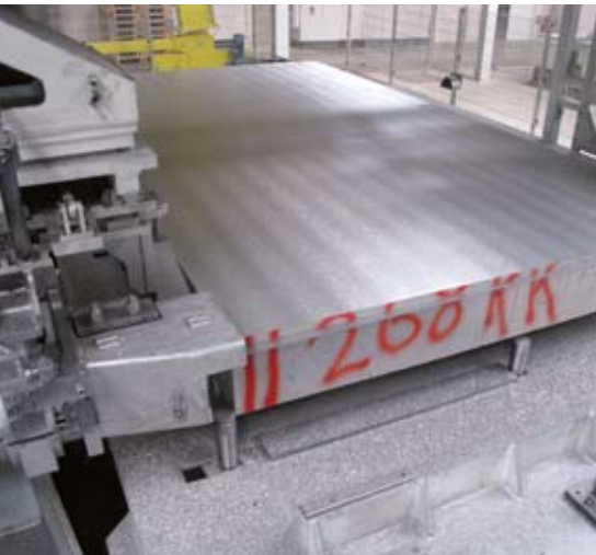
Plate sawn to rough dimensions
