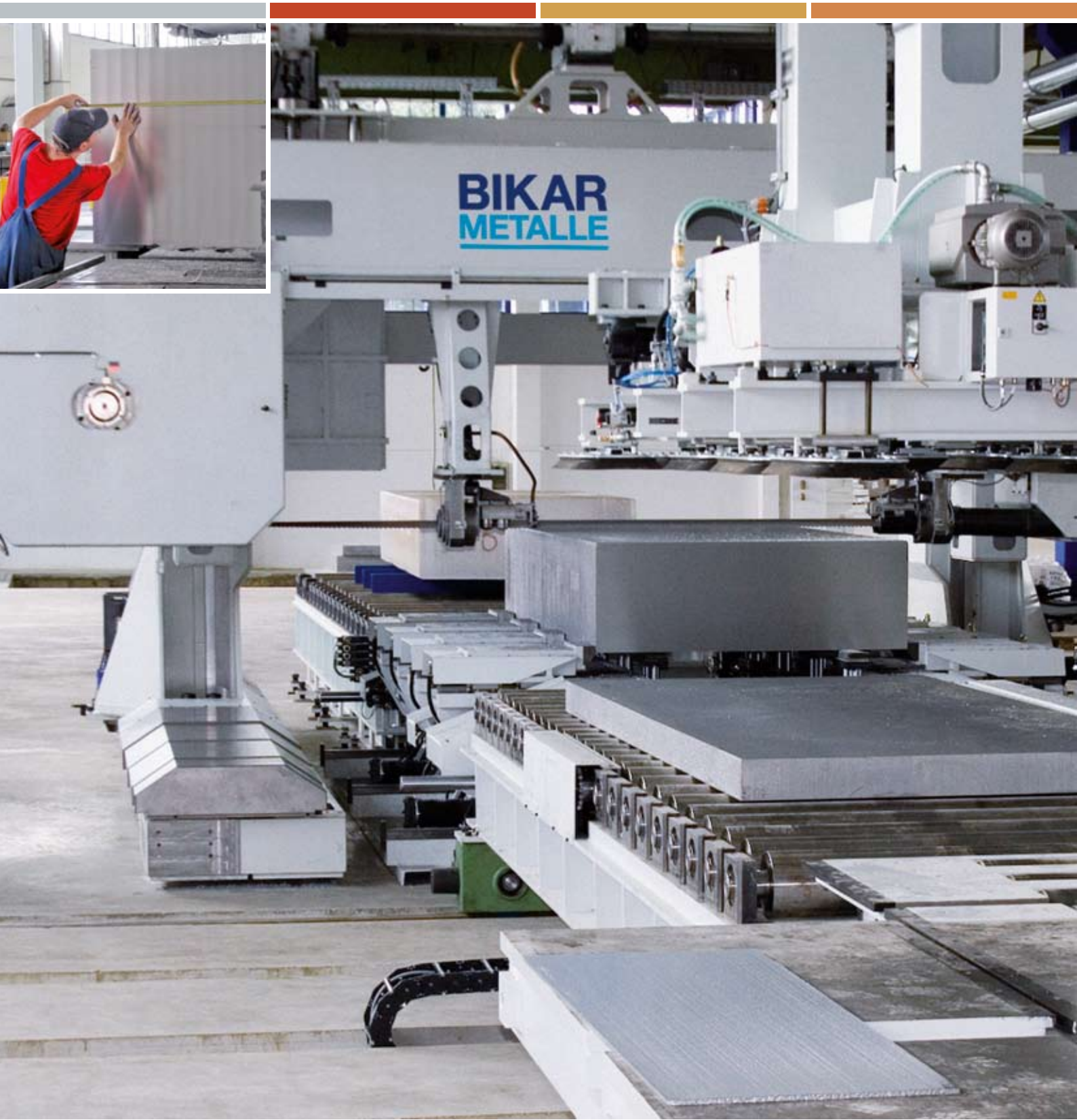
Saw plant for plates with unit weights up to 35,000 lbs
