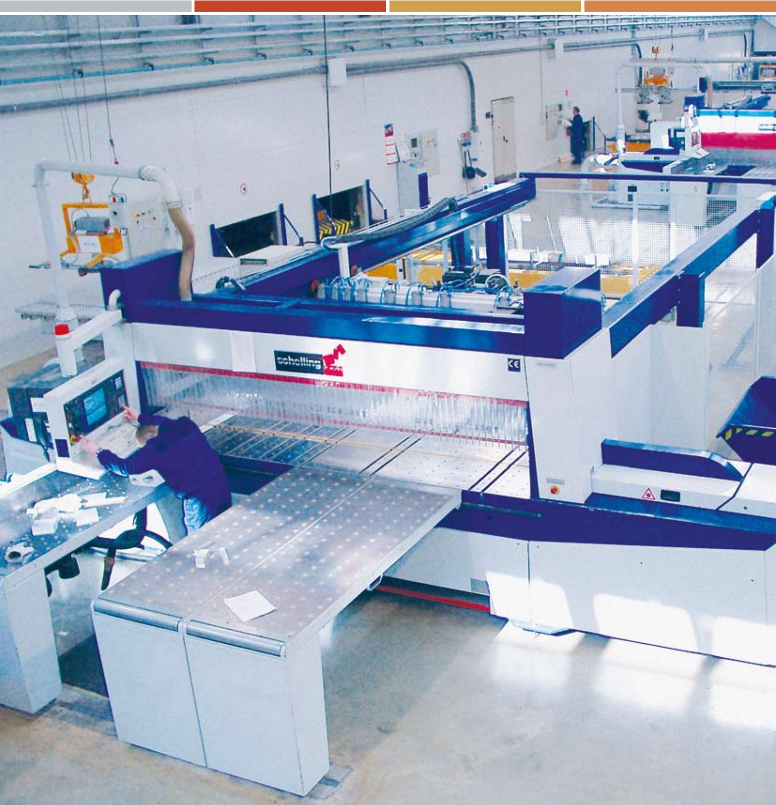
Precision circular saw for rolled plates
