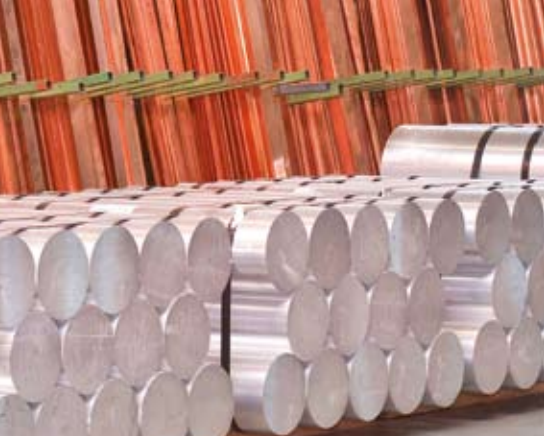
Cast ingots up to 23.6 inches in diameter
